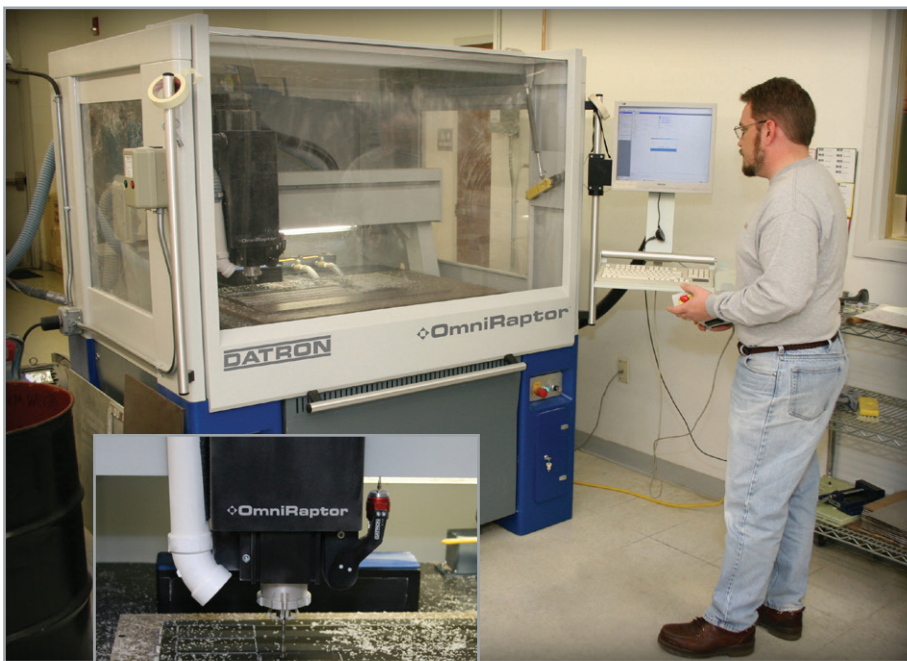
QC Drilling machine operator, Ron Twardosky, runs small flat Lexan parts on the DATRON M8 machining system — a run of 15 is not uncommon.
