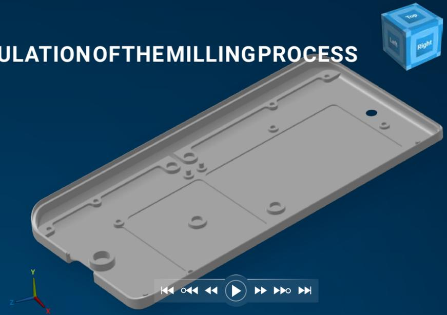
By means of the DATRON next simulation, the paths of the milling process can be calculated, taking into account the tools that are already assigned in the machine. Finally, the workpiece is visualized in 3D. You can now preview the entire machining process in the simulation and check in advance whether the desired milling result is achieved. You can zoom, rotate and push the virtual workpiece around with your fingertips at will.
