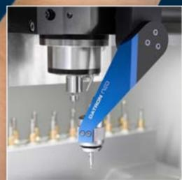
The correct setup of the workpiece, including establishing a zero point for orientation in the machining area, is one of the basic requirements for excellent machining results.
