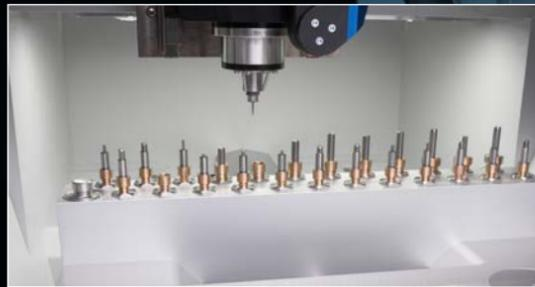
**24-station tool magazine with integrated tool-length sensor**
