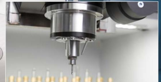
**2 kW spindle and minimum-quantity coolant system**
