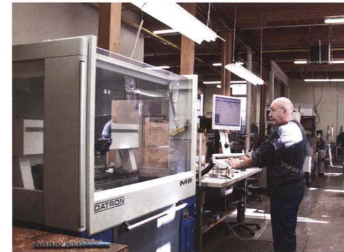
John Dionne, machine shop manager at Burkart-Phelan, uses a Datron M8 machining center with a 60,000-rpm spindle and an integrated 4th axis to mill intricate parts on a solid gold flute.
