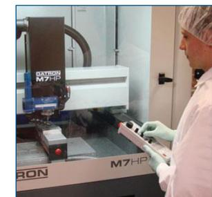
The DATRON also leaves a superior surface finish, Arnold notes. “With the incredible accuracy that the DATRON provides, it eliminates tool marks typical of 3-D molds that are cut with a step-over.”
