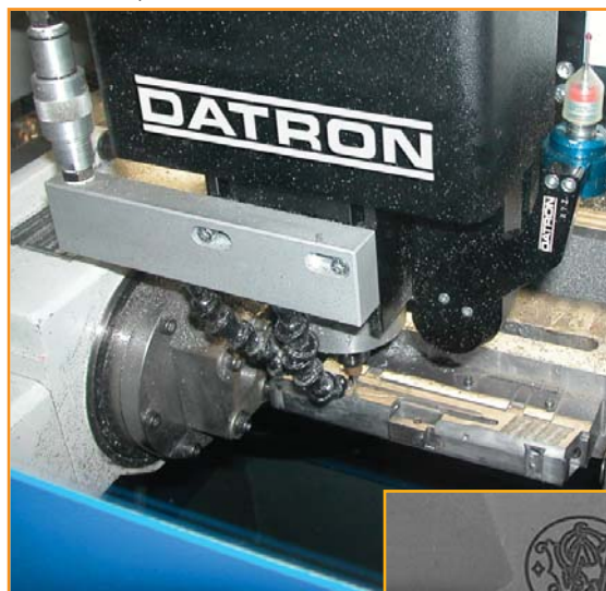
A 3D Probe detects and compensates for surface variance while flexible Integrated Workholding is designed to accommodate every gun in your product line (including long guns).
