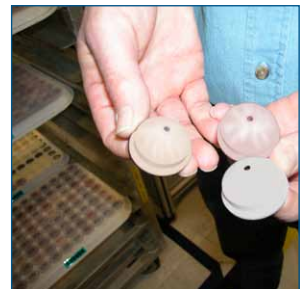
Photo 3: While the range of color and marbling from one section of lava to another is no problem, the varying density and growth properties even within a single blank poses a real machining and part uniformity challenge.
