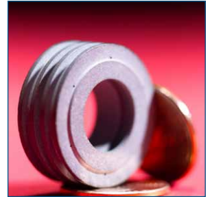
Photo 1: A finished Hypertherm plasma cutter swirl ring with .011" holes micro-drilled in lava on a DATRON high speed machining center.
