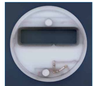
Step 2: Parts are secured with the vacuum fixture so that all of the detailed features that appear on the back can be machined.
