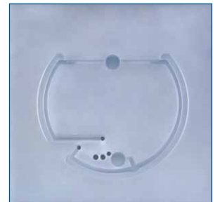
Step 1: Blanks milled from sheet of military-grade cast acrylic.
